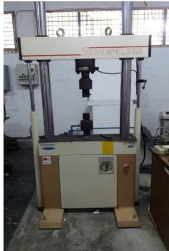
Fig. 3. Universal Testing Machine (UTM) Shimadzu Servopulser 10 kN
