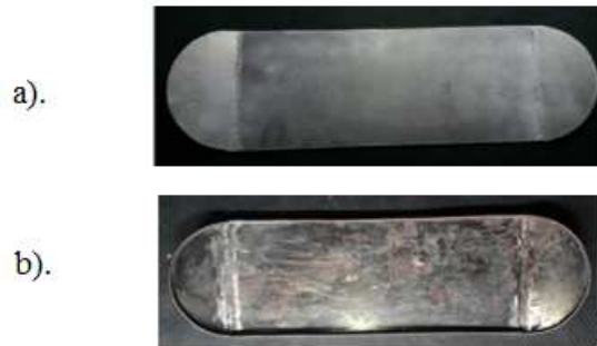
Fig. 5. Skateboard mold on commercial standar: (a) top cover, and (b) base
